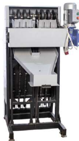
Figure 5. Nut sheller for industrial use Reference Source: [21].
