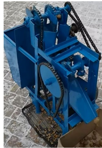
Figure 4. Mechanized device for cracking walnut shells (for non-industrial production volumes) Source: [21].
