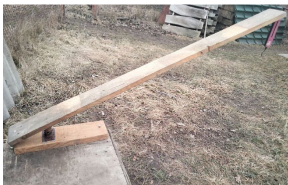
Figure 6. Laboratory equipment for determining the strength characteristics of walnut fruit
